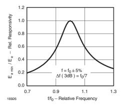
Figure 5. Frequency Dependence of Responsivity
