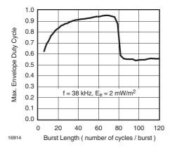
Figure 9. Max. Envelope Duty Cycle vs. Burstlength
