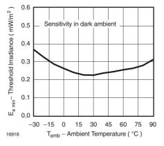
Figure 10. Sensitivity vs. Ambient Temperature
