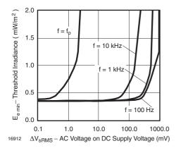
Figure 7. Sensitivity vs. Supply Voltage Disturbances
