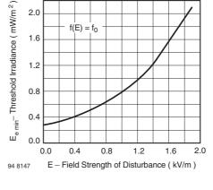
Figure 8. Sensitivity vs. Electric Field Disturbances
