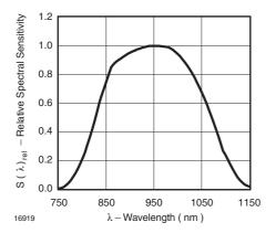
Figure 11. Relative Spectral Sensitivity vs. Wavelength
